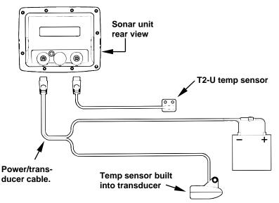
Sonar unit with secondary temperature sensor. Primary temp sensor is built into the transducer.
